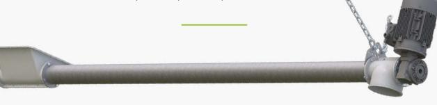
Tunetanken Transport Conveyors are specially developed for efficient transportation of grain and grinded materials such as flour, minerals, soybean meal, rapeseeds and beans. Transport Conveyors can be used in both of two modes: horizontally or inclined at an angle up to 45°. Transport Conveyor has a speed of 400 rpm and a flange pipe in lengty varying from 3 to 12 meters.
